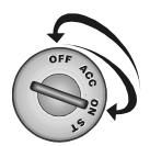
Turn ignition to "run" position, then turn to "off" position. Press and release the Valet switch within 10 seconds. The Status LED will light steady if you have entered Valet Mode, and it will go out if you exited Valet Mode.
